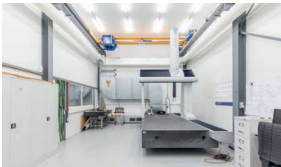
DEA Global – die moderne 3D-Messmaschine in Grenchen
